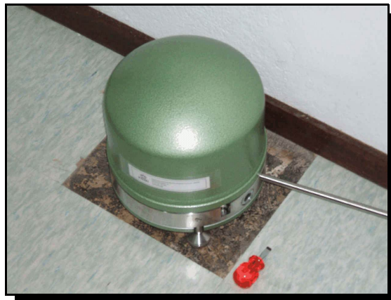
One of the STS-2 seismometers installed in the SSS Islands.
